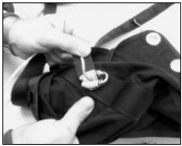
is covered by the black loop. The collapse line should exit the bridle between Kevlar and the link should lie as shown [Fig. 6]
