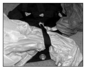
Pass the large loop at the end of the bridle through the canopy bridle attachment loop, then pass the entire assembly, starting with the pilot chute handle [Fig. 2] through the large loop in the bridle.
