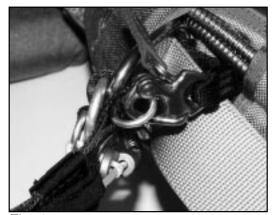
Attach the snap shackle to the main riser RSL ring and inspect routing. The RSL shackle must not interfere with the operation of the 3-Ring System. [Fig. 4]
