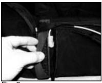
Insert top of release handle into loop on container, then mate handle to container. [Fig. 2]
