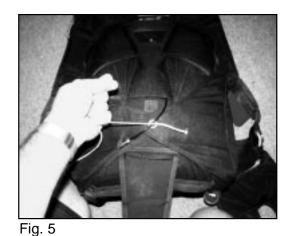
Close side flaps and pin. Remove pull-up cord. [Fig. 5]
