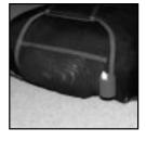
Insert folded main pilot chute in the spandex pouch. [Fig. 6]
