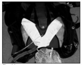
Distribute the remaining 3-4 ft of bridle on top of the #1 closing flap.[Fig. 25]
