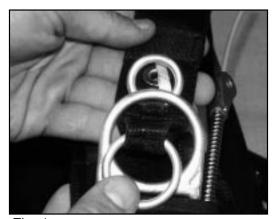
With the rings of the riser facing forward, pass the large ring on the end of the riser through the large harness ring from above. Fold it back toward the canopy and risers. [Fig.1]
