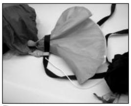
Pass the large loop at the end of the bridle through the canopy bridle attachment loop, then pass the entire assembly, starting with the pilot chute handle through the loop in the bridle. [Fig. 7]
