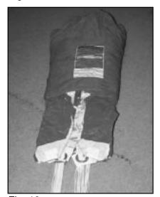
Cocoon the canopy to the width of the reserve freebag mouth lock. Canopies cocooned wider may increase bulk. [Fig. 10]
